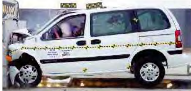
Frontal crash test of Chevrolet Venture
