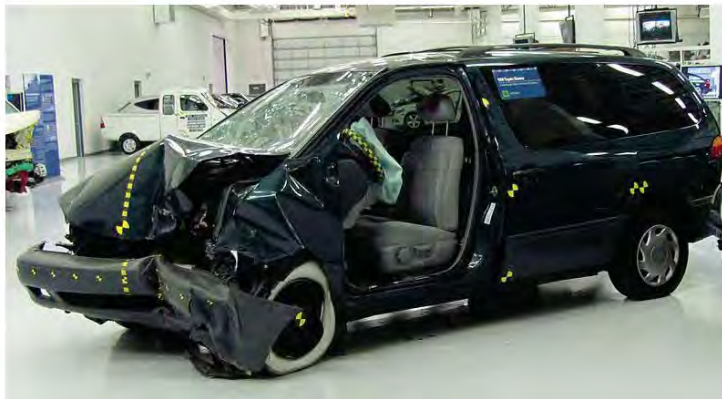
Offset frontal crash test of 1998 Toyota Sienna
