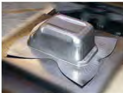
Deep-drawing of blank metal sheet (source: ThomasNet)
