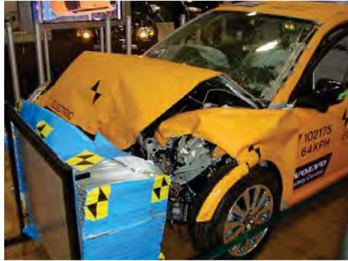
Frontal crash test of Volvo C30
